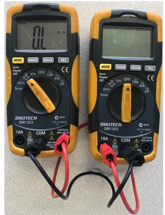
Fuse is blown: "0.L" indicates discontinuity
