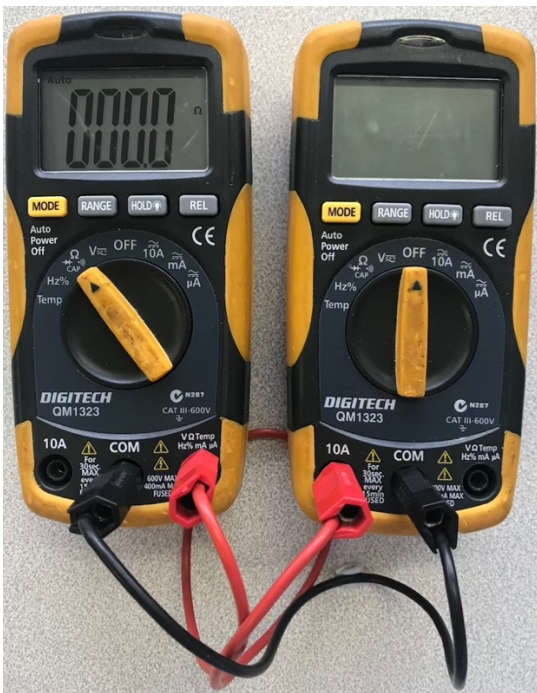
Fuse is OK: 0 resistance ( \Omega ) = continuity
